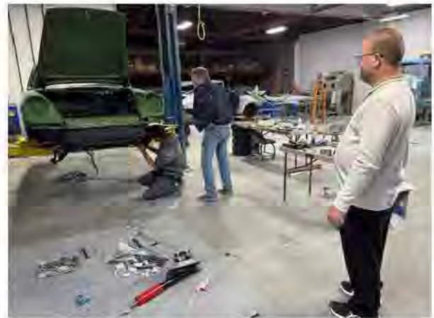
All the suspension parts were on the car except for the last rear shock and hub assembly that I had taken to have a bearing pressed into.
