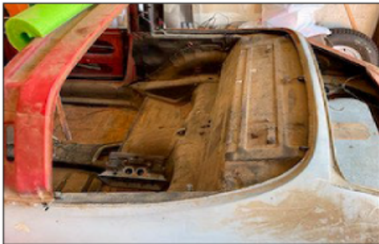
The Parcel Shelf in the rear window had lots of rusted pinholes and apparently this shelf is different on a Targa than a Coupe. And no one sells a new Targa version. So the welder just cut out an area, recreated it and welded it back in.
