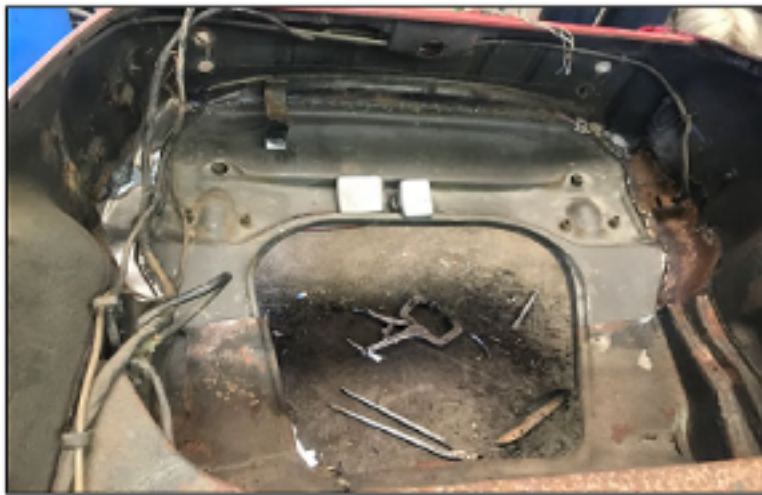
Replacing the U-shaped fuel tank front support, but the welder cut the old one below the factory spot welds as well as the new one in the same place to match them but keep the factory welds.
