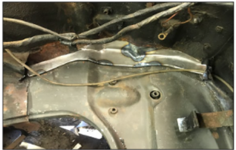
The front left corner of the same piece which will be below the battery. The windshield washer fluid container support is on the right.
