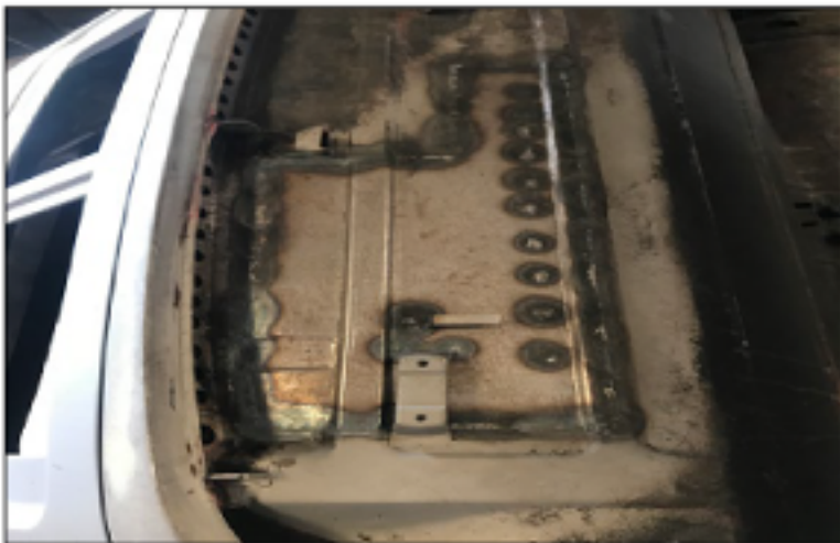
The Parcel Shelf in the rear window had lots of rusted pinholes and apparently this shelf is different on a Targa than a Coupe. And no one sells a new Targa version. So the welder just cut out an area, recreated it and welded it back in.
